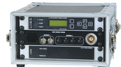
L9203 Receive Station Receiver (Top) Connection Panel (Middle) Triax Interface Unit (Bottom)
