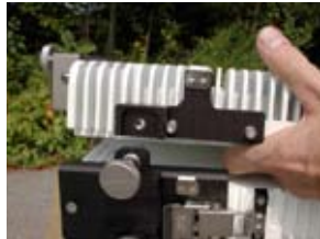
Figure 2-7 Removing Unit from Stack with Universal Bracket
