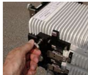
Figure 2-6 Captive Screws on Universal Bracket
