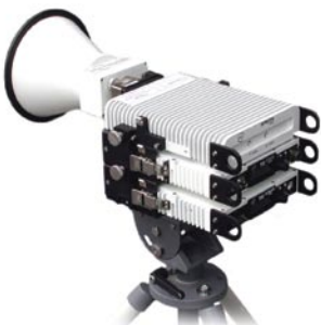
STRATA TCU, 2 GHz TXU, and 2 GHz HPU mounted on Universal Stackable Brackets with MegaHorn Antenna
