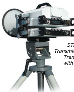
STRATA 3 to 13 GHz Transmitter Unit (TXU) with MegaHorn Antenna
