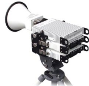
STRATA TCU, TXU, and HPU mounted on Universal Stackable Brackets
