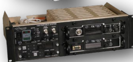
STRATA TXU & TCU (2 GHz Only) installed in the VPS Portable Van Shelf with Outdoor Unit
