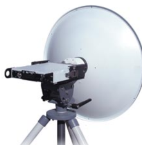
STRATA Receiver Unit (RXU) with 2' (60 cm) diameter antenna
